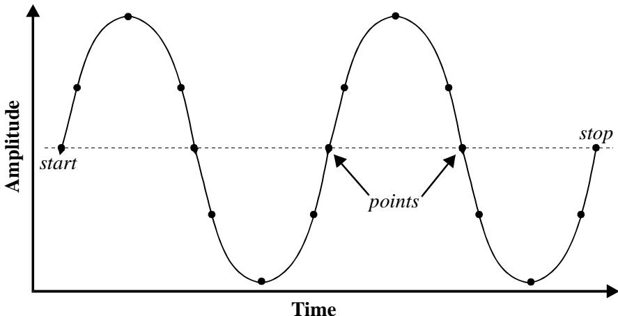
Points are individual “samples” of the waveform’s amplitude at specific times. The locations of points at intersections of the X (time) and Y (amplitude) axes define the shape of the waveform. The greater the number of points, the greater the potential resolution when representing a waveform.
